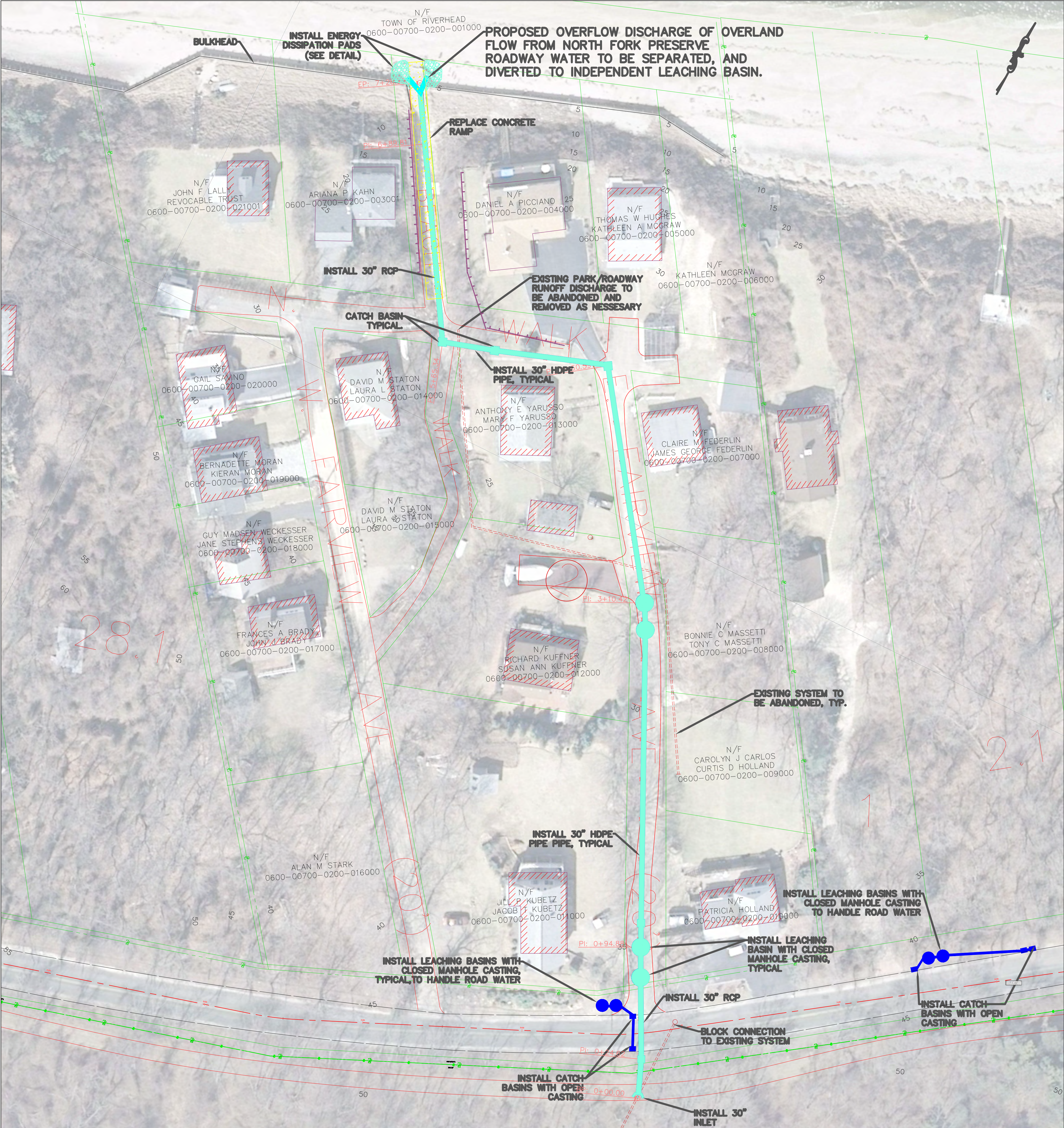
PIPE SYSTEM #1 SCALE 1" = 30'
